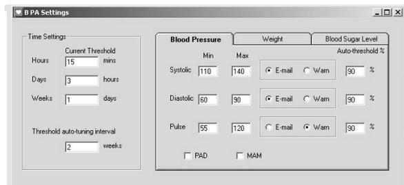
Figure 1: GUI screen allowing thresholds to be set and percentages of values that need to be within threshold before they automatically adjust based on the threshold auto-adjust time.
